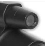
Infra-red illuminators, or IR illuminators, are common to night vision. The IR light greatly enhances the performance of the NightStar while remaining almost totally invisible to the naked eye. The IR illuminator on the NightStar is located underneath the front lens, next to the battery compartment.
