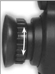
To focus the NightStar, first you will need to adjust the diopter. Simply turn the diopter clockwise until it stops. Then, while looking through the diopter at an object, slowly turn the diopter back counter clockwise until the grain in the image is sharp.
